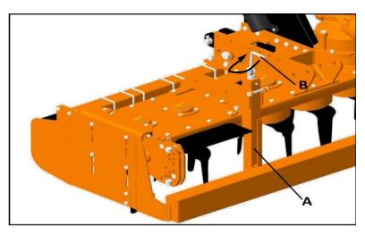
It is recommended to set the bar position at 4-5 cm higher compared to the position of the roller on the ground.
