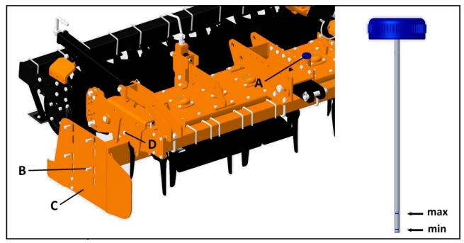
If the mark is below the minimum, fill up oil till the correct level is restored.
