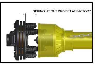
An adjustment can be done, however, when the clutch slipping is too frequent, which means that the calibration is too low. In this case, the tightening of nuts over the compressed springs will give
