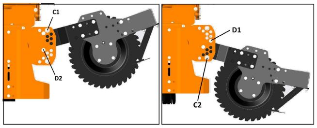
The roller can be left in floating configuration, free to follow the ground contour, by positioning the adjusting pin (D2) in a hole lower to position (E) immediately below to the connecting arm, or by removing it altogether.
