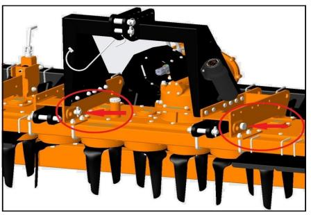
If, after the adjustment, the PTO shaft is still too long, the operator will have to uninstall and adapt it by shortening the transmission tubes, according to the instructions of the use and maintenance manual of the driveline Manufacturer.
