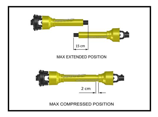
A driveshaft too long may cause structural damages to the tractor and machine. If the driveshaft is too long, it may be adapted by removing it and shortening the tubes according to the instructions provided by the Manufacturer in its use and maintenance manual.
