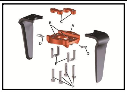
The blade housing is clamped to the rotor flange by means the screws and screws stopping, and hosts the two blades, locked in the housing through the stopping forks and the snap pins.
