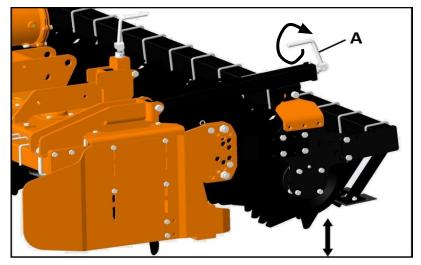
The position of the roller frame relating to the swinging arms affects the adjustment of the working depth.
