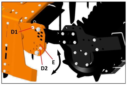
This configuration can be useful in case the machine meet an obstacle during operation, allowing the machine to overcome it without damaging the roller, thanks to the swinging arms, and obtaining a nearly uniform levelling of the ground.
