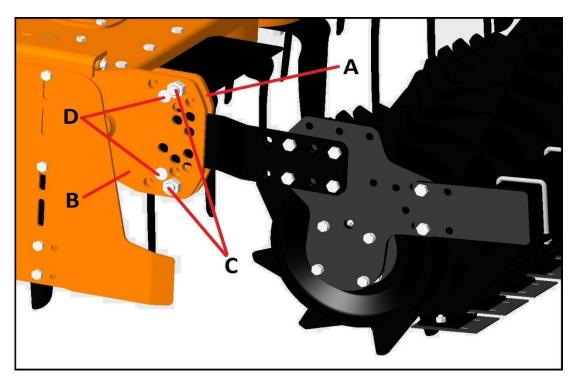
Operator can adjust the roller height in eight different positions, by inserting the two adjusting pins (D) into the holes immediately above and below the roller's swinging arms, according to the desired working height.
