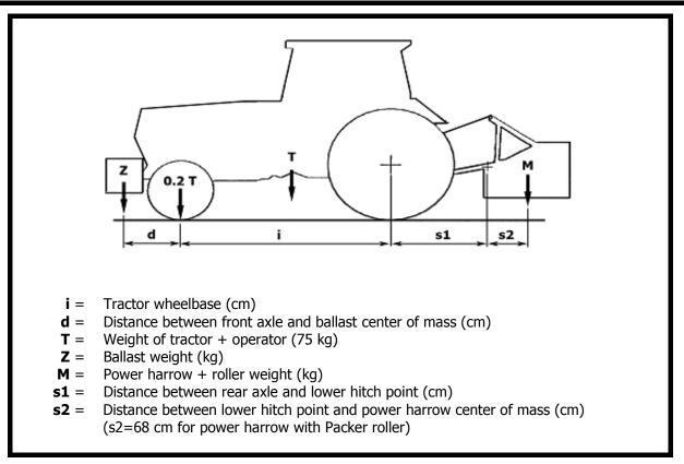
If the machine is combined with other machines (fertilizers spreaders or seeders), the ballast check must be done considering:
